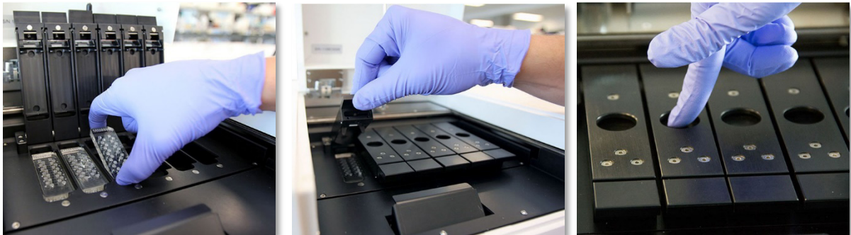
Figure 89: Proper orientation of cartridges when placing them into the Digital Analyzer. Close the magnetic clips gently and be sure to push down on the metal plate above the cartridge after the lid is closed to ensure the cartridge lays flat.
