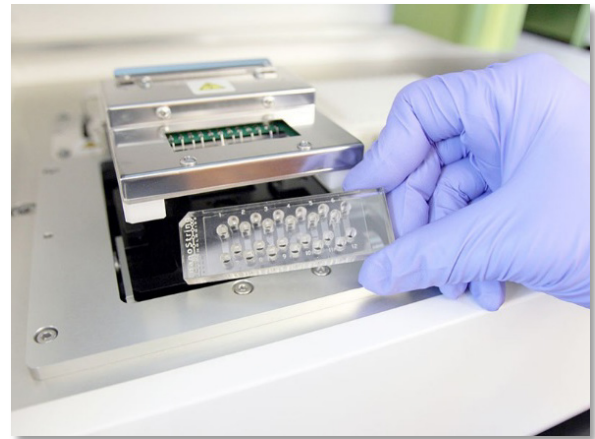
Figure 25: Insert an unused cartridge into the Prep Station in the orientation shown.
